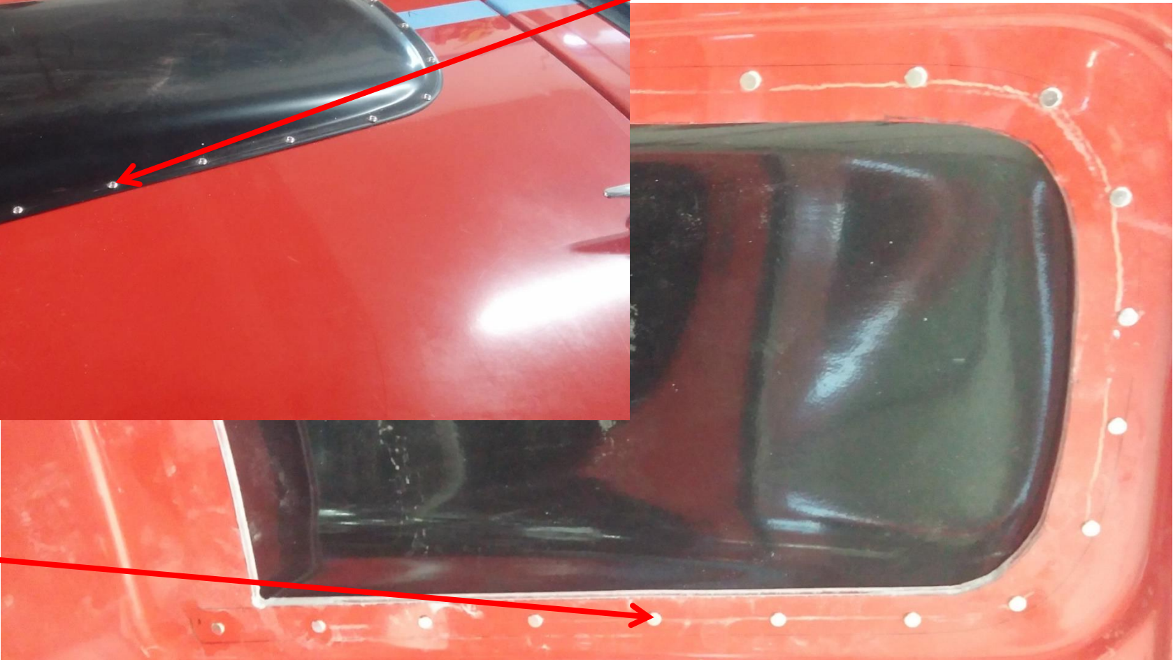
Stainless Socket head cap screws in place of pop rivets
