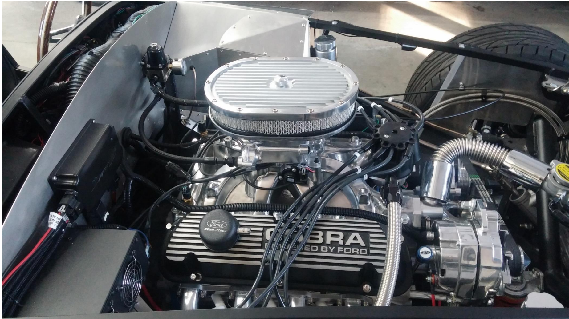
Engine with 90% of electrical and plumbing dressed out
